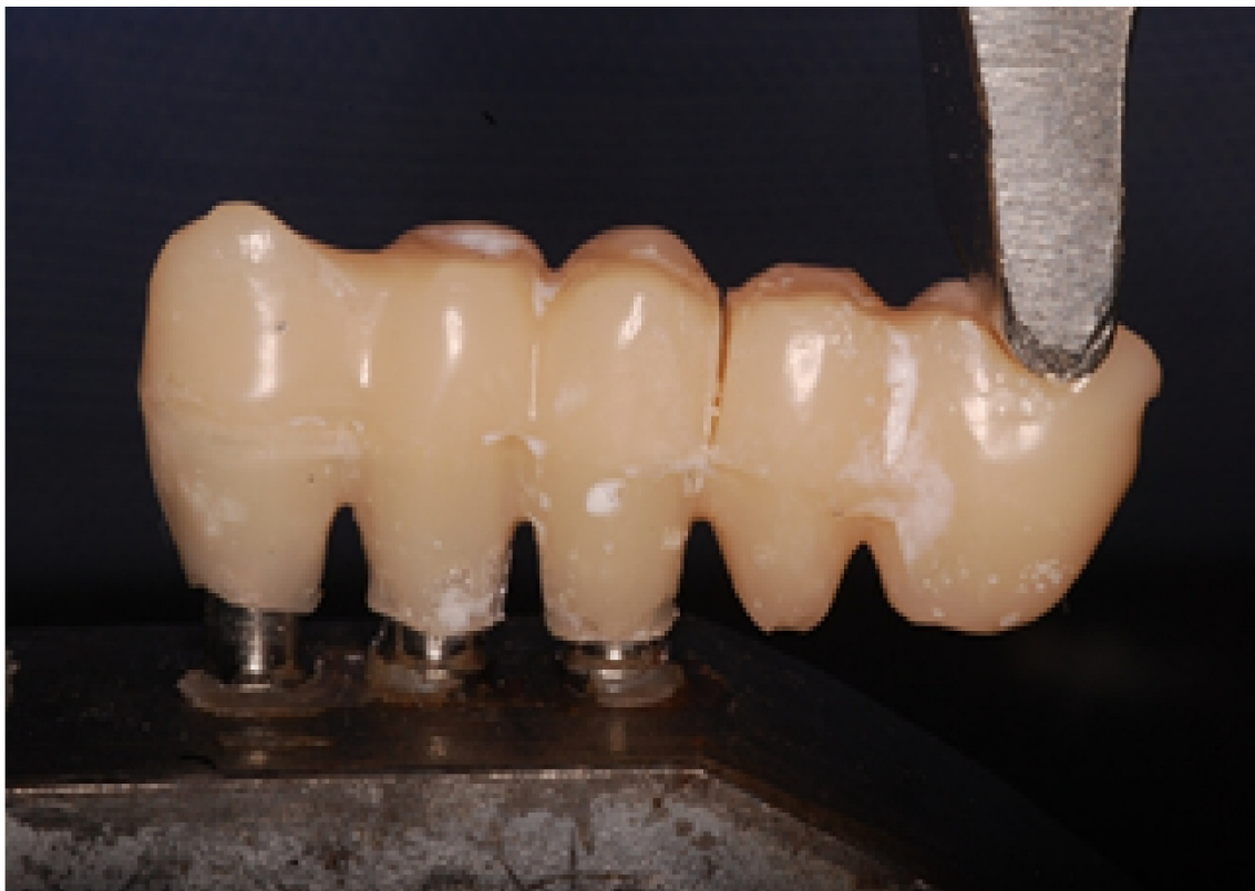
Figure 3. Moment of specimen fracture when tested in the universal testing machine.
